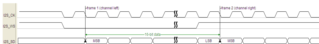
Figure 19-16. I2S Phillips standard timing diagram (DTLEN=00, CHLEN=0, CKPL=1)
